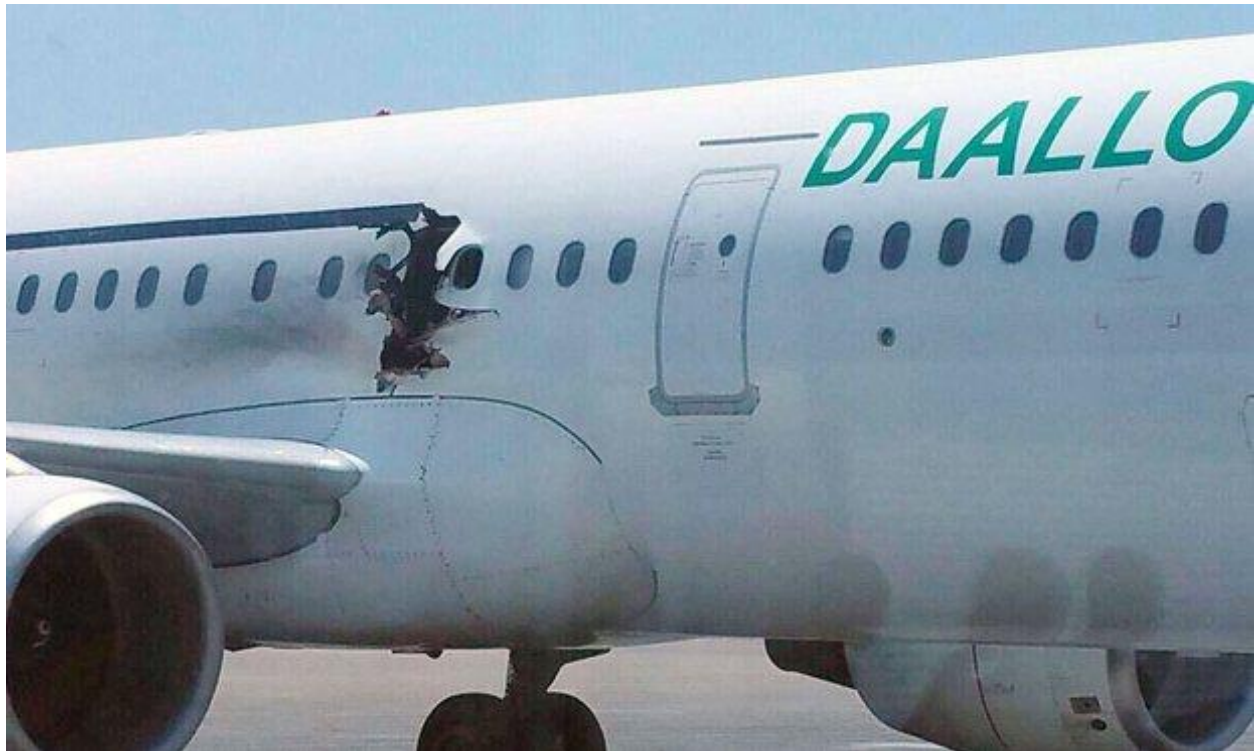
Fig. 1: Dalo airplane that exploded mid-air. You can clearly see one meter hole in the side of the airplane torn by the explosion
